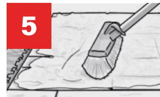
**5** Sweep off excess GATOR POLYMERIC SAND from the paved surface, first with a hard-bristle broom, then a soft bristle broom. Joints sand level, must be at least 1/8 inch (3 mm) below top of paver's surface or 1/8 inch (3 mm) below the chamfer.
