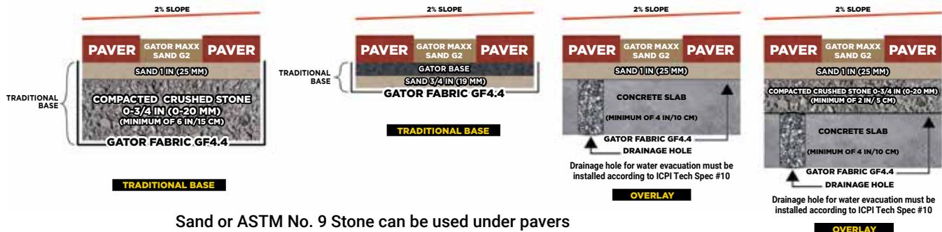
Sand or ASTM No. 9 Stone can be used under pavers
