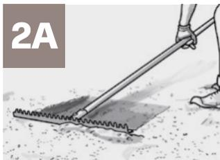
**A** Ensure a slope of at least 2% away from any structure, such as a house.
