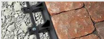
Gator Edge Flex and Rigid are made with 100% Polypropylene Copolymer. This gives it great strength as well as providing greater flexibility. We have a Rigid model which is ideal for straight applications and a Flex model that can be used for all curved applications such as walkways, paths, entrances, etc. Both the Rigid and Flex can be locked together with the "Twist & Lock" connection system. The Rigid could be transformed in a partial Flex by cutting the bridge support.
