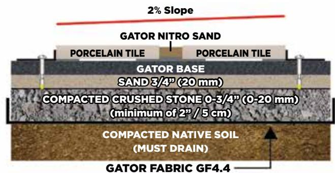
Sand or ASTM No. 9 Stone can be used under Gator Base panels
