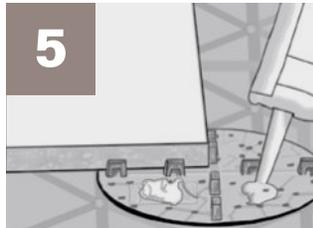
Gator Spacers should receive a generous amount of Alliance polyurethane XP glue on each quadrant. Install the Porcelain Tile on the Gator Spacer, apply pressure or tap the tiles with a rubber mallet at all corners. This will ensure that the tiles are adhering to the Gator Spacer. The Gator Spacer will be left in the tile installation permanently, ensuring proper alignment and stability of your project for years to come.
