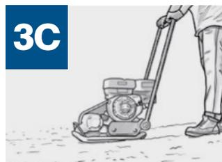
**C** Shower the complete sand area to aid into the compaction step. Using a hand compactor and/or plate compactor, compact the 3/4" (19 mm) of sand until you obtain a final height of 1/2" (13 mm) of compacted sand. The final area should be smooth.
