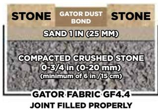
Sand or ASTM No. 9 Stone can be used under stones
