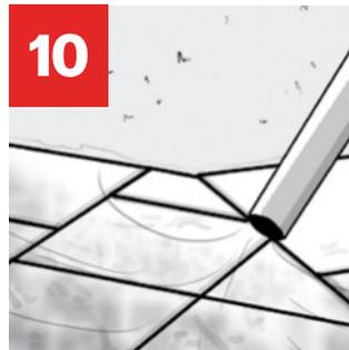
**10** Use a leaf blower to remove any excess water remaining on the paver pores and crevices. This blowing action is necessary to help remove any remaining GATOR POLYMERIC SAND residue left on paver surfaces from the previous steps.
