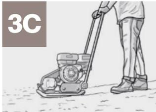
**C** Water the sand prior to using a hand compactor and/or plate compactor, compacting the layer of sand until you obtain a final height of 1/2" (13 mm) of compacted sand. This compacted surface should reflect the final tiled surface.
