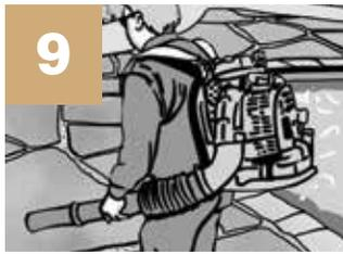
**9** Use a leaf blower to remove any excess water remaining on the wet cast or natural stone pores and crevices. This blowing action is necessary to help remove any remaining GATOR DUST residue left on wet cast or natural stone surfaces from the previous steps.
