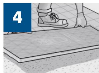
Make sure to install the Gator Base on the extended excavation area (total excavation should be 6" (15 cm) wider on each side than the final paved area or 12" (30 cm) for a seat wall or fire pit). Start laying the Gator Base units while ensuring locking of the tongue & groove system. This will guarantee the panels' stability when the pavers or slabs are laid down. Trim any visible curves or protruding angles using a utility knife.
