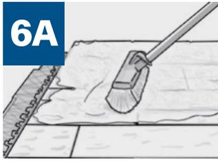
**A** Spread GATOR MAXX **G2** with a hard-bristle broom. Make sure the GATOR MAXX **G2** completely fills the joints. Do not use other materials in the joints. Leave a layer of GATOR MAXX **G2** on the surface to aid in the vibrating and consolidation of GATOR MAXX **G2** into joints.
