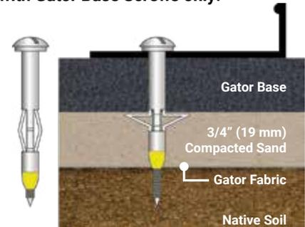
Fastening Gator Edge with the Gator Base Screw through the Gator Base reinforces the outside perimeter, creating a strong lateral support. Gator Base Screws are a required component on any Gator Base install.
