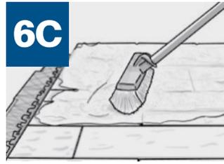
**C** Sweep off excess GATOR MAXX **G2** from the paved surface, first with a hard-bristle broom, then a soft-bristle broom. Take care to leave the height of the polymeric sand at least 1/8" (3 mm) below the top of the stone or 1/8" (3 mm) below the chamfer of the paver.
