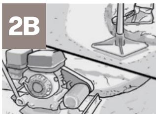
**B** The native soil needs to be compacted using a plate compactor or hand tamper.
