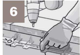
Install Gator Tile Edge on the Gator Base using Gator Base Screws, make sure that Gator Tile Edge rests firmly against the tiles. Use Gator Base Screws at every second hole.
