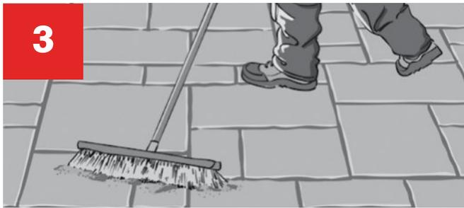
Sweep off excess GATOR MAXX G2 from the paved surface, first with a hard-bristle broom, then a soft-bristle broom. Take care to leave the height of GATOR MAXX G2 at least 1/8 inch (3 mm) below top of paver's surface or 1/8 inch (3 mm) below the chamfer.
