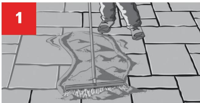
Spread SUPERSAND **G2** with a hard-bristle broom. Make sure the SUPERSAND **G2** completely fills the joints. Do not use with other materials in the joints. Leave a layer of SUPERSAND **G2** on the surface to aid in the vibrating and consolidation of SUPERSAND **G2** into joints. For textured or pre-finished surfaces, we recommend to remove all the sand from the paver or slab surface prior to using the plate or roller compactor.
