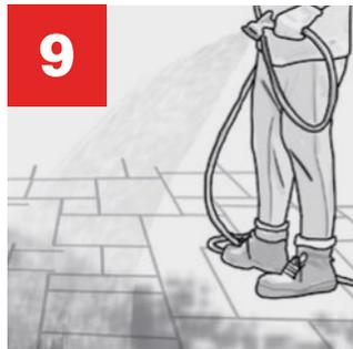
**9** Shower and rinse simultaneously, so as to eliminate any GATOR POLYMERIC SAND residue. Any residue should go directly into the paver joints. However, stop showering when you see water retention on the paver joints. Wait no longer than 2 to 3 minutes. Proceed to STEP 10.
