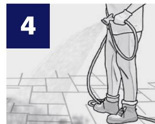
**4** Shower for a minimum of 50 seconds for 4,6 sq. m. or until the EUROSTONE BOND repels the water and the water starts to accumulate over the polymeric sand joints.
