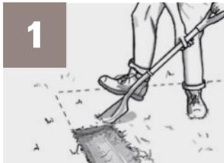
Excavate the new Gator Tile area. The depth required is calculated by adding Porcelain Tile height, Gator Base, compacted sand, plus any soft organic material that has to be removed. Excavate the perimeter an extra 6" (15 cm) wider on all sides than the finished tile area requires.
