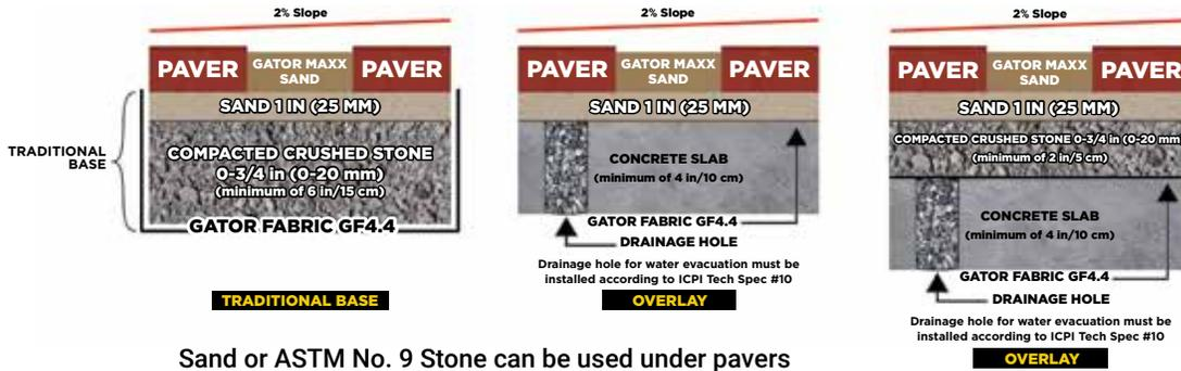
Sand or ASTM No. 9 Stone can be used under pavers
