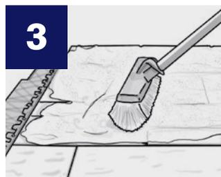
**3** Sweep off excess EUROSTONE BOND from the paved surface, first with a hard-bristle broom, then a soft-bristle broom. Take care to leave the height of EUROSTONE BOND at least 3 mm below top of natural stone pavers surfaces.
