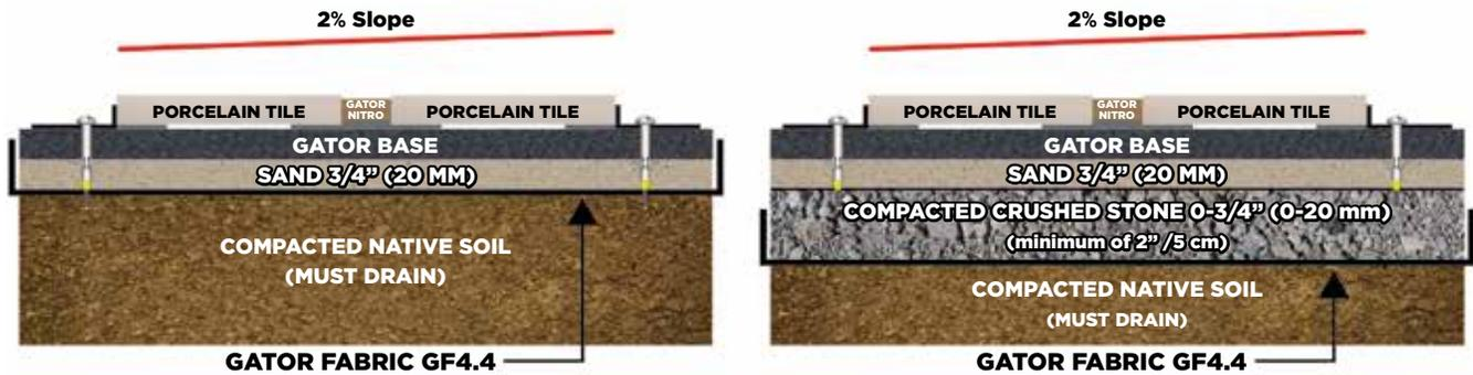
To use with 3/4 inch (20 mm) outdoor porcelain tile only. Sand or ASTM No. 9 Stone can be used under Gator Base panels.
