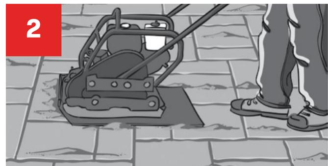
Vibrate the SUPERSAND **G2** into the paver joints using a vibratory plate compactor. A rubber pad is recommended. A roller compactor is best for slab installation. Joints sand level must be at least 1/8 inch (3 mm) below top of paver's surface or 1/8" (3 mm) below the chamfer. It is best to compact in several directions to ensure there are no air gaps or voids in the joints. Repeat steps 1 and 2 to ensure joints are filled and consolidated. Narrow joints require more care to completely fill.
