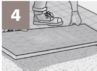
Make sure to install the Gator Base on the extended excavation area (total excavation should be 6" (15 cm) wider on each side than the final tiled area). • Start laying and staggering the Gator Base units ensuring Gator Base interlocks with the tongue & groove system.
