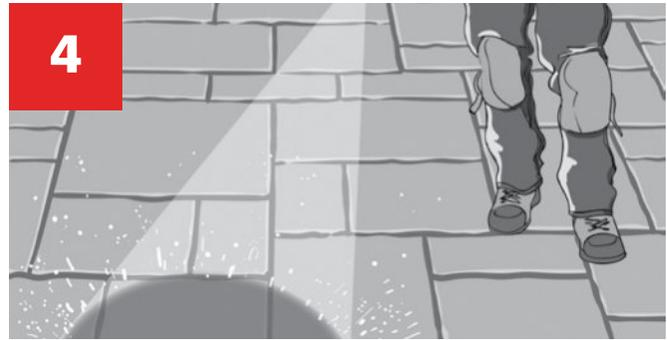
Shower for a minimum of 30 seconds for 30 sq. ft. (3 sq. m.) or until the SUPERSAND G2 repels the water and the water starts to accumulate on the joints.
