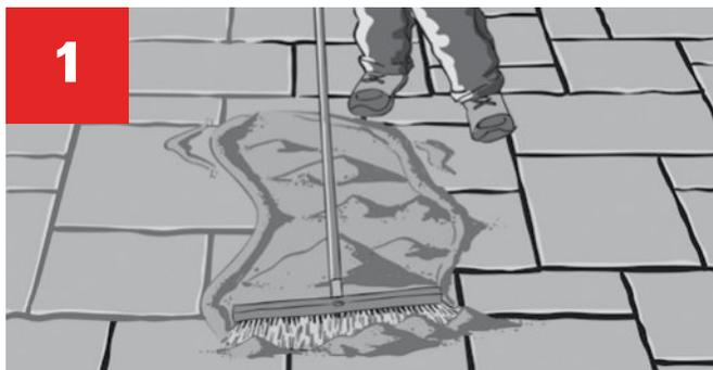
Spread GATOR MAXX **G2** with a hard-bristle broom. Make sure the GATOR MAXX **G2** completely fills the joints. Do not use with other materials in the joints. Leave a layer of GATOR MAXX **G2** on the surface to aid in the vibrating and consolidation of GATOR MAXX **G2** into joints. For textured or pre-finished surfaces, we recommend to remove all the sand from the paver or slab surface prior to using the plate or roller compactor.
