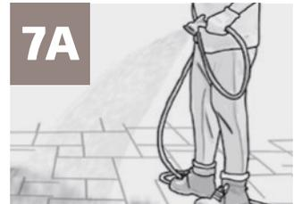
**A** Ensure the entire area to be jointed is thoroughly wet. If the surface is dry or temperature is high, more water will be required to avoid staining of the surface when spreading the GATOR NITRO JOINT SAND.
