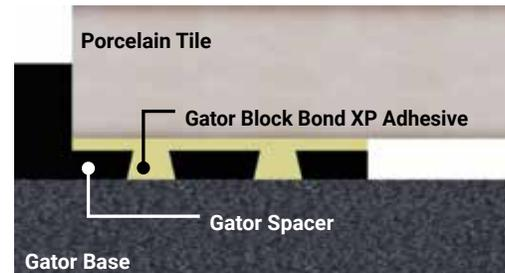
Gator Block Bond XP penetrates into the concave holes, adhering the Porcelain tile to the Gator Tile Spacer, then hardens. This allows the tile to minimize any horizontal or vertical movements.
