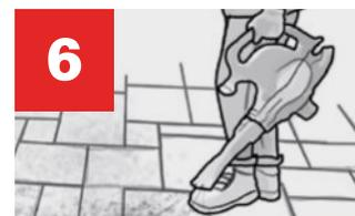
**6** Use a leaf blower to remove all remaining GATOR POLYMERIC SAND residue from the paver surface.
