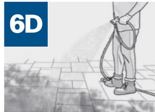
**D** Activate GATOR MAXX **G2** by showering 30 sq.ft. (3 sq.m.) section for 30 seconds, starting at the lowest point. Once all the sections are activated, rinse off any debris that is on the total paver surface.
